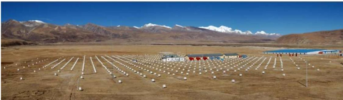
Those gamma rays reaching the Earth's surface can be detected in arrays like these ones in the above image found 14,000 feet above sea level on a Tibetan plateau.
